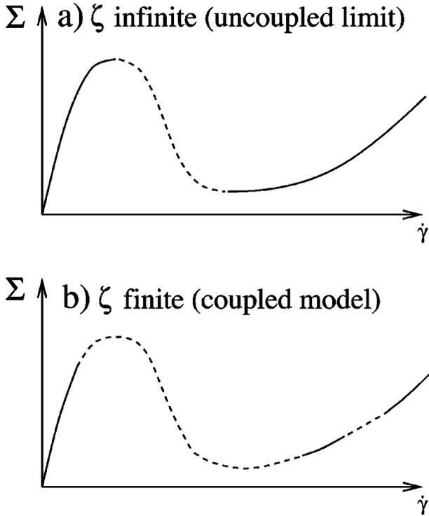
FIG. 7. Sketch of the unstable (dashed) region of a mechanical instability (a) decoupled from or (b) coupled to concentration. As discussed in the text, concentration coupling broadens the region of instability and can sometimes cause a new region of instability to develop in the high shear rate branch (see Fig. 3).
