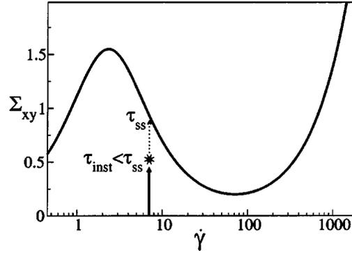
FIG. 9. Cartoon: homogeneous start-up flow going unstable at time  $\tau_{\text{inst}}$  before it can reach the intrinsic unstable constitutive curve at time  $\tau_{\text{ss}}$ .
