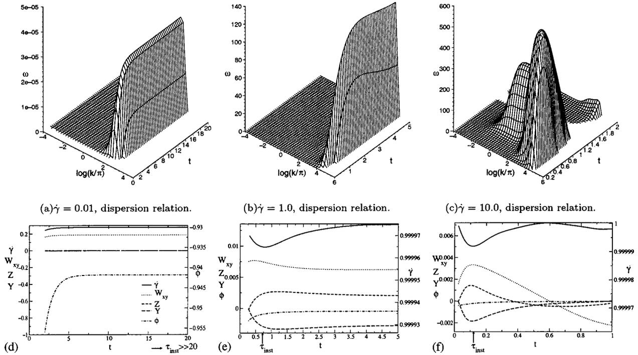
FIG. 12. Type B instabilities (a), (d) and type A instability (b), (c), (e), (f) in a type II system: time-dependent dispersion relation (top) and eigenvector (bottom) for a coupled model in which all parameters assume the experimental values of Table I, *except*  $D$ , which is reduced by a factor of  $10^5$ . The concentration  $\phi=0.11$ . The arrows in (e), (f) show the time at which the instability first becomes measurable [the instability occurs beyond the time window of (d)].
